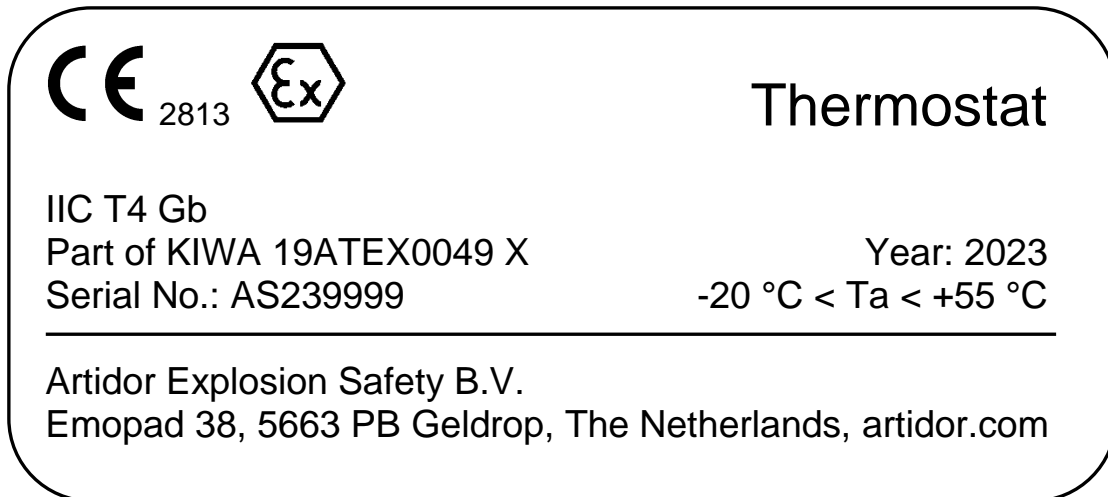
Figure 3. Example of the label of the thermostat as "Simple apparatus"
